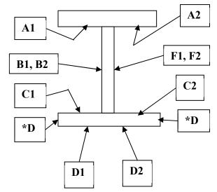
\*D areas are only included when flange thickness is one inch (1") or greater. \*D areas are only included when flange thickness is one inch (1") or greater.
